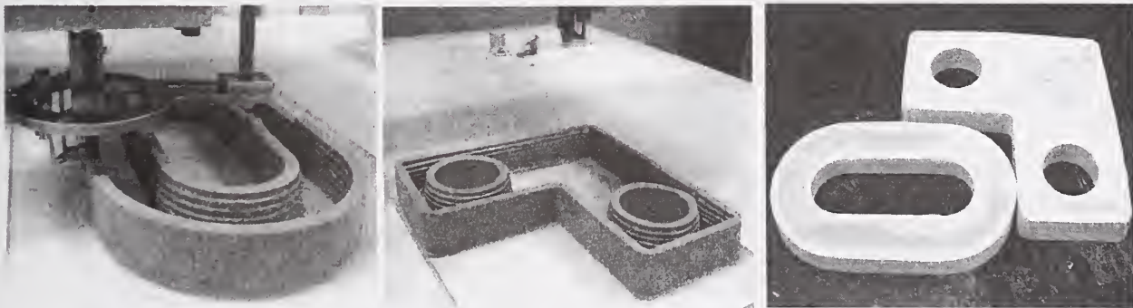
Figure 8. Sections with cavities made with CC and filled with concrete (largest dimension in these figures is 10")
